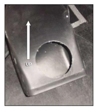
Figure 8a. Four inch hole cut in Volvo duct.
